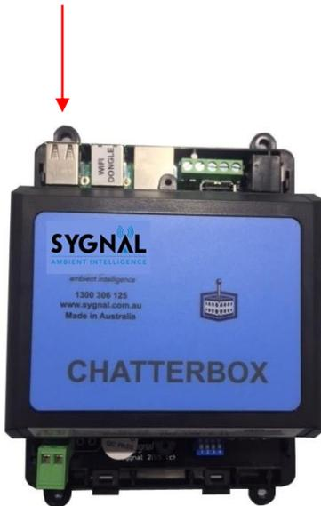
**Figure 7** – Connecting via Ethernet cable
