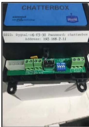
*Figure 1 – Label on chatterbox shows MAC address, IP address and password*
