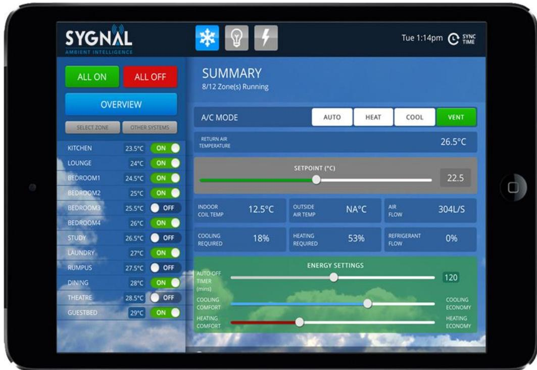
Figure 12 – Example of Sygnal Climatepoint multi-zone temperature control user interface on an Ipad Mini.
